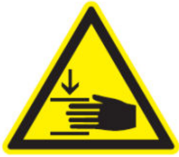
Image 8. Danger of squeezing
