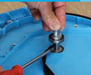
**4** The strap and the pin can be easily pulled back. Then take the pin out of the loop of the strap so the strap can be pulled through the axis.
