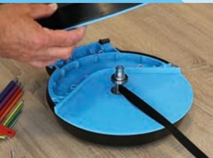
**3** Take a pointed tool, such as a flat screwdriver and pull the pin through the axis. Due to the training activity it can be tight. Hold the device and press tight.
