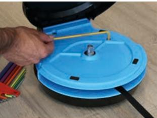
**2** After removing the discs you have access to the two hexagonal screws that hold the two metal sideplates together. Open both screws and take off the top sideplate to get access to the band axle.
